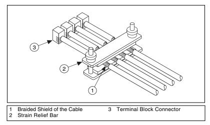
Figure 22. Required Cabling for CE Compliance
